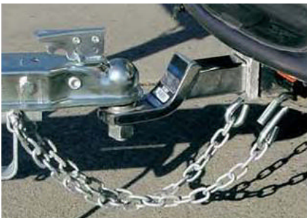
Fig 3: Proper attachment of the safety chains is essential to trailer safety. Note how the safety chains are crisscrossed.
