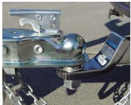
Fig. 2: Coupler on ball with latch in proper lock position.
