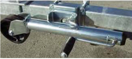
Fig 4: Swing jack in traveling position.
