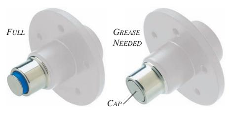
The hub is full of grease when the blue Autocheck® ring is visible. The cap on the end of the blue ring contains messy grease overflow.
